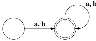
. Automate reconnaissant  $c_1 L_1 \cup \dots \cup c_i L_i, c_j \in \Sigma, L_j \in \Sigma^*$
